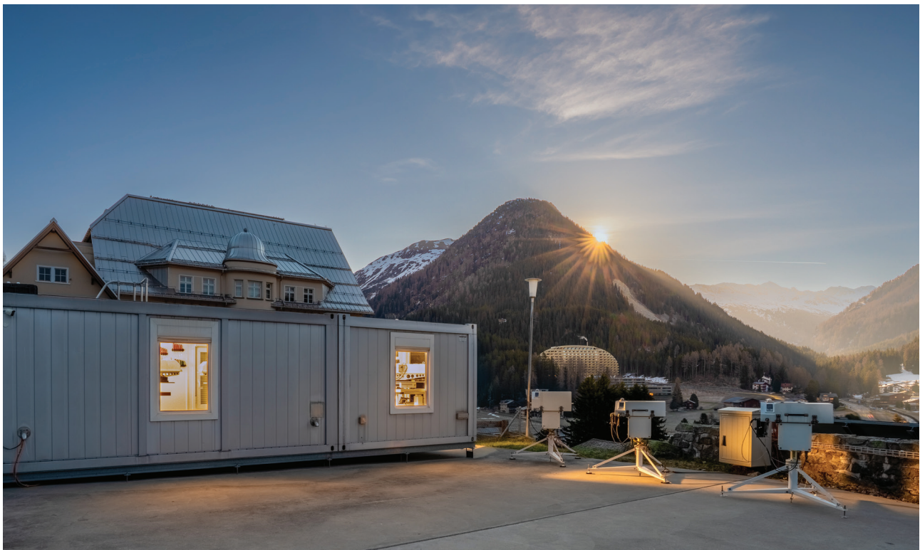
Figure 6: The instruments in 2026 with the 3 Brewer spectrophotometers (outside) and the 3 automated Dobson spectrophotometers (in the container) on the measurement platform at PMOD/WRC Davos. Source: Fabrizio Vignali, PMOD/WRC.
