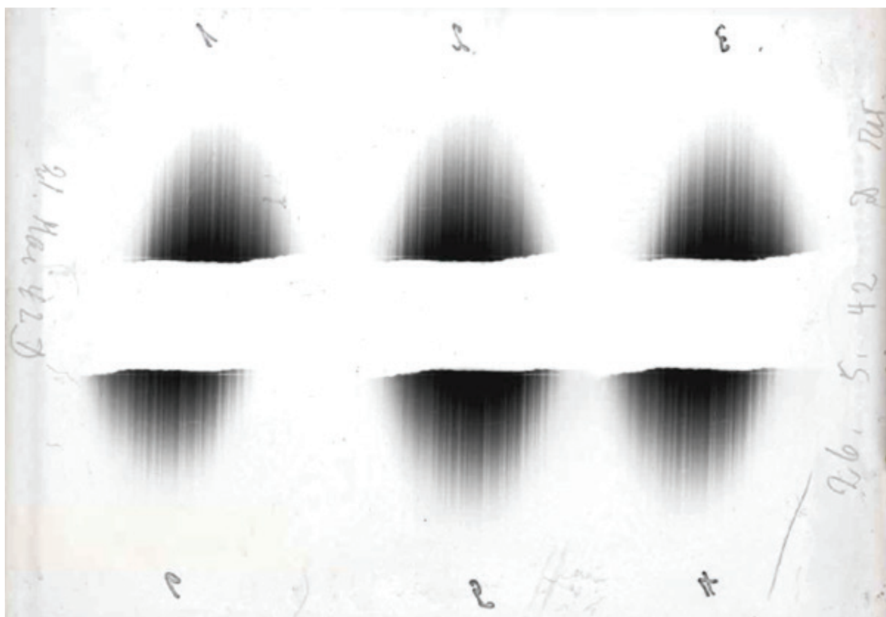
Figure 7: Photographic plate of March 21, 1942. Each “half-ellipse” is a solar spectrum dispersed by the Féry prism. The 6 spectra are repeated exposures at different solar zenith angles during the same day. The vertical dimension represents light intensity (darkening of the photographic emulsion), and the horizontal dimension represents UV wavelengths. The optical density of the plate darkening was measured at specific wavelengths pairs and compared with a known UV source reference. The TCO was computed from the difference in darkening between the two wavelengths. Source: MeteoSwiss Archives.
